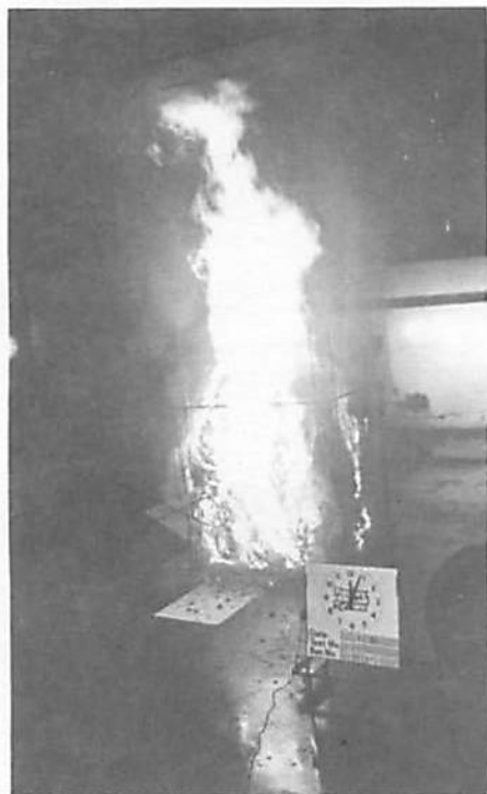
In the test for combustibility, 15 foot high stacks of (defective) RL01 and RL02 disk packs were completely engulfed in flames in less than five minutes.
