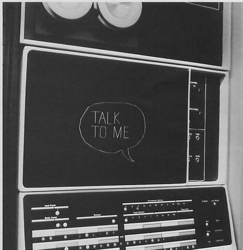
USERS CAN "TALK" to their Digital Equipment Corporation PDP-12 computers through DIAL-2, the updated version of its systems software. DIAL-2 (Display Interactive Assembly Language) uses the computer's built-in display.
