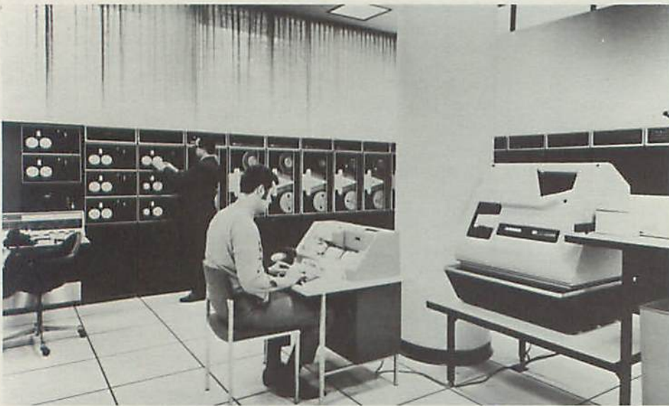
A section of Dataline Systems Limited's computer center in Toronto shows part of their PDP-10, the largest ever delivered by DEC. Dataline time-sharing customers will use the PDP-10 for scientific and design problem solving, accounting analysis, and for data banks for storing statistical and financial data.
