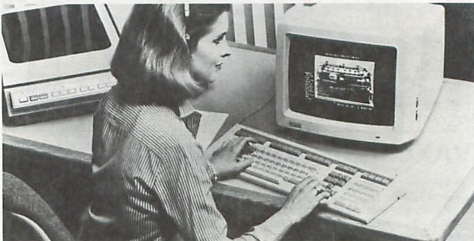
IVIS, multimedia "video learning station" combines the Professional 350 with a hardware-software option package that integrates video images from videodisc or other sources, computer generated text and graphics, and synchronized, two-channel sound.
